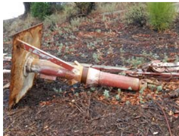
Winch Stored In Contractor Staging Area (assumed LBP)
