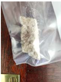
HMS-M17224-104A Pool Area Plaster
