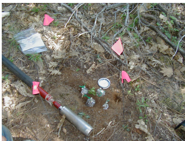
Figure 10 Soil Sample Plot Showing Soil Corer, temperature, and in this Photo, Nitrogen Sampling Bags
