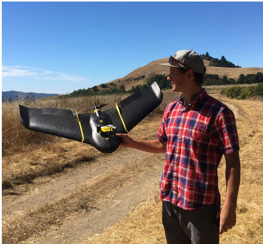
Figure 6 The Ebee® Fixed wing UAV
