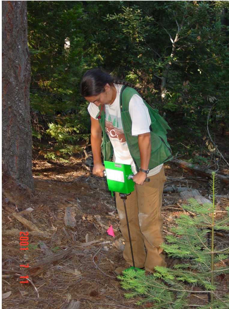
Figure 12 A Soil Penetrometer Being Used in the Field to Assess Compaction in Forested Ecosystems.
