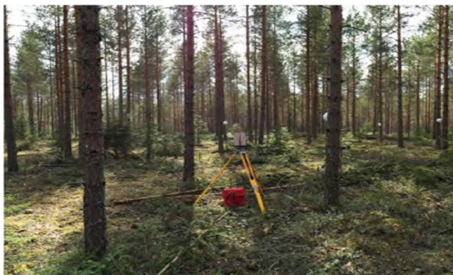
Figure 13 A Terrestrial LiDAR Unit Used to Capture Post Treatment Data in a Treated Forest Stand
