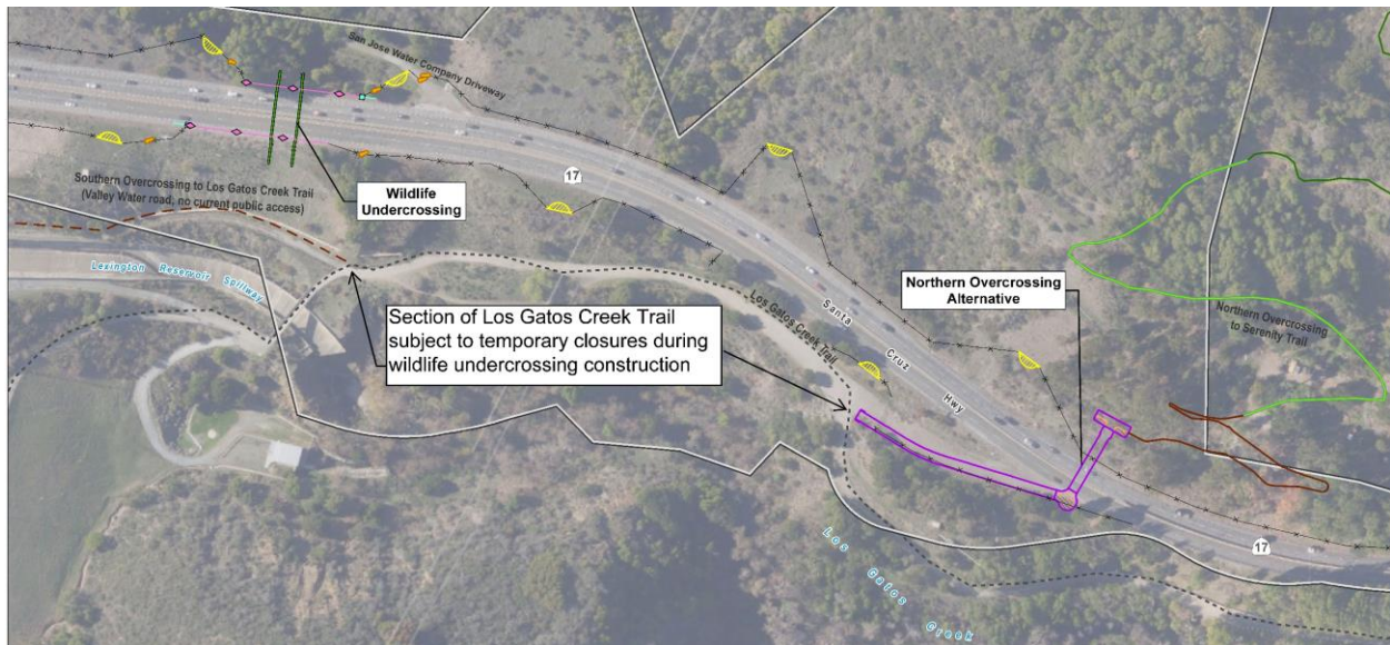
Figure 2.2.3-1: Detail of Potential Los Gatos Creek Closure Area (see Figure 1.4-1 for complete legend)
